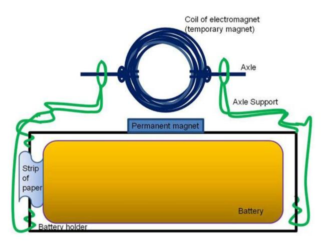
**Figure 5.** This drawing shows how to connect the electromagnet and its axles, the permanent magnet, axle supports, battery, and its paper switch to form a simple electric motor.
