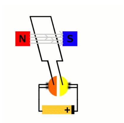
**Figure 2.** This animation shows the direction the loop of wire (the electromagnet) will rotate, based on Fleming's Left Hand Rule for Motors. (ExplainThatStuff.com, 2008.)
