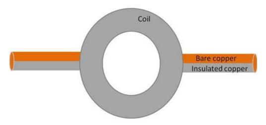
**Figure 4.** This drawing shows the parts of the axles to strip of insulating material.
