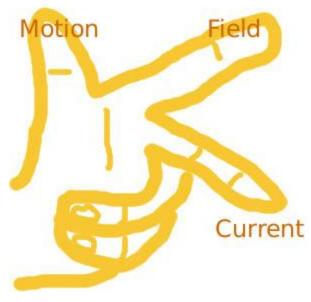
**Figure 1.** This drawing shows Fleming's left hand rule for motors. (ExplainThatStuff.com, 2008.)
