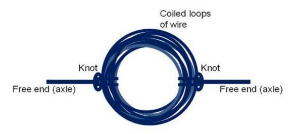
**Figure 3.** This drawing shows how the electromagnet and the axle that it spins on will look when it is formed.
